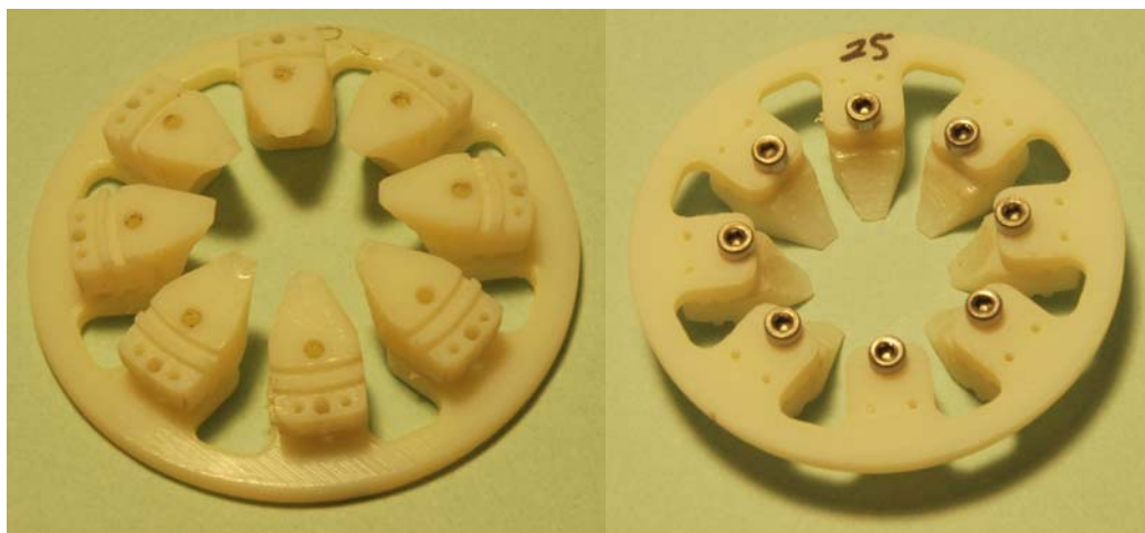
Figure 3.7: Shoes mounted on annular base plate (left), shoes constrained onto annular base plate using M2 screws (right).
